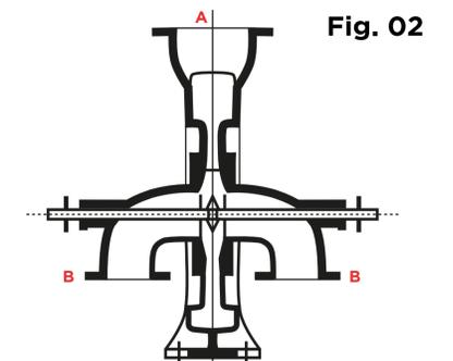
The turbine may be placed at any height, less than 25 feet, above the tail-race, the fall below the wheel being rendered available by suction pipes descending from the central discharge orifices into the tail water. Frequently this admits of the placing of the Vortex in a position more convenient for the application of the power than at the bottom of the fall.
